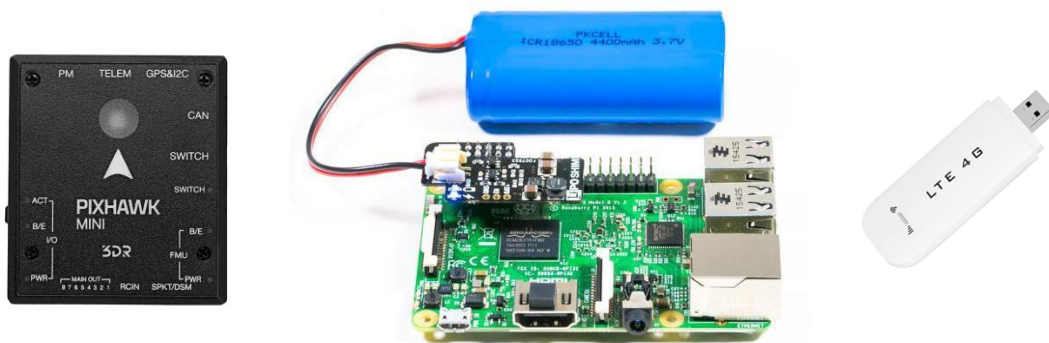
Figure 12: Components of telemetry module to be integrated in the drone
