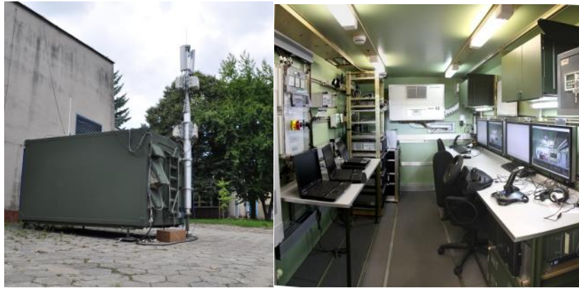
Figure 9 Control station used in FP7-SECURITY TALOS project founded by European Union. Contains HMIs for mission management and operation of two UGVs.
