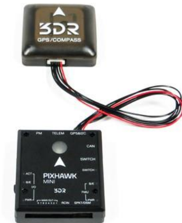
Figure 13: GPS module connected to Pixhawk mini
