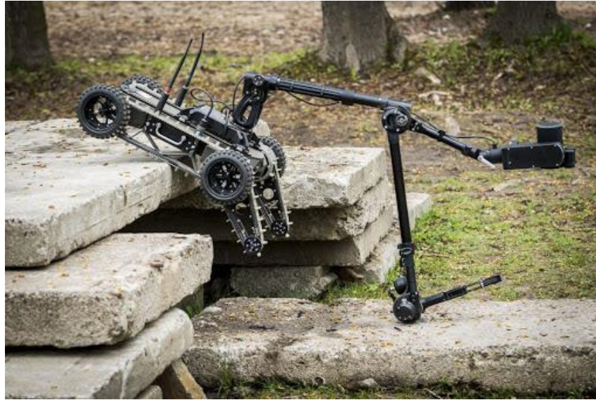
Figure 30: PIAP GRYF utilizing manipulator's range for advanced movement technique
