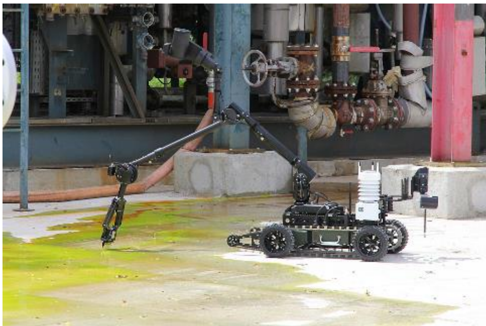
Figure 7 PIAP Gryf® robot taking samples, with additional payloads on the back of UGV.
