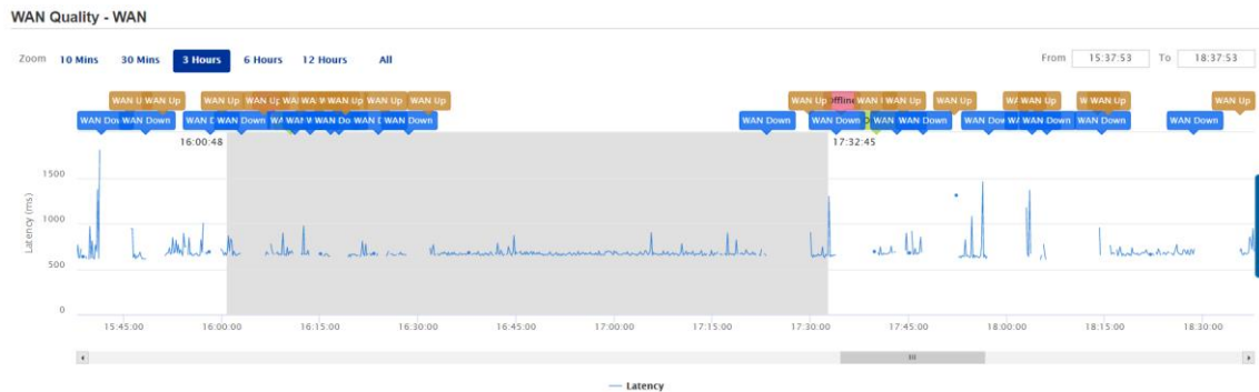
Figure 27 - Timeline graph of the satellite link latency during the deployment test
