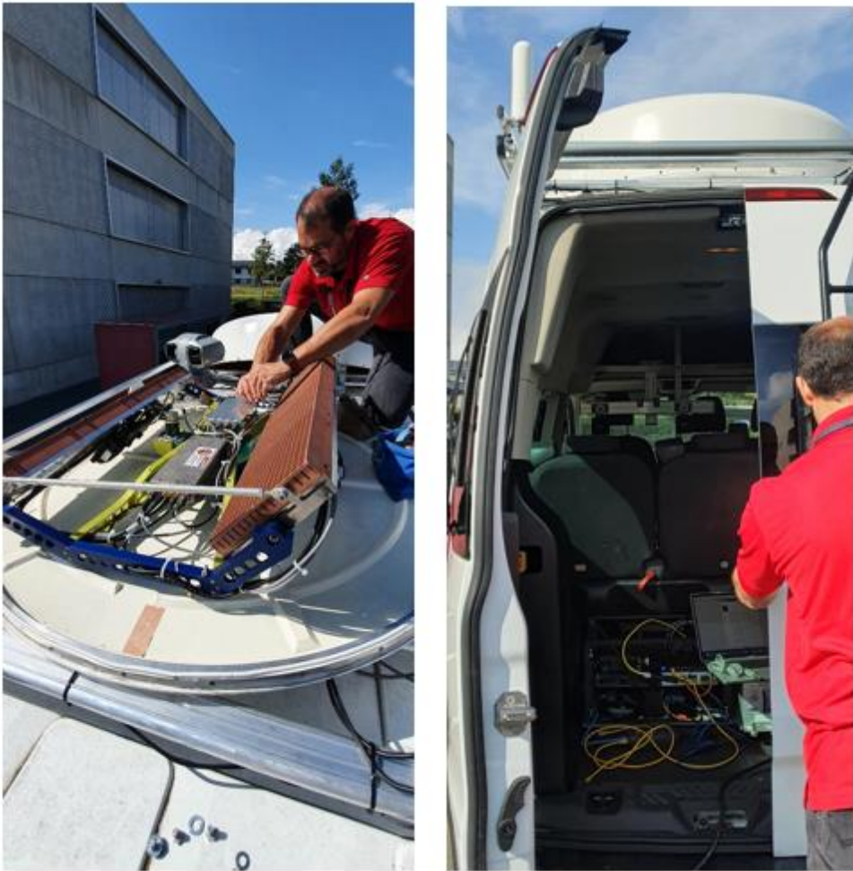
Figure 12 - KaLMA antenna mounted on the roof of the Viasat Land Vehicle
