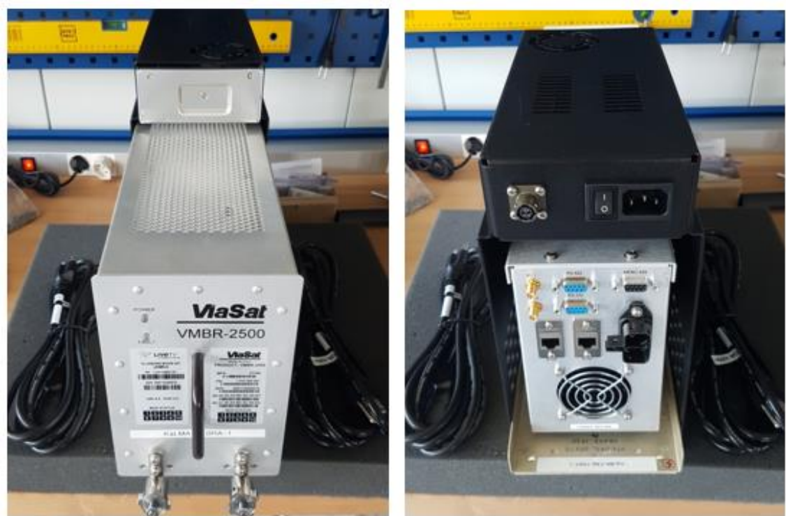
Figure 14 - Viasat mobile terminal (modem) and ACU power source
