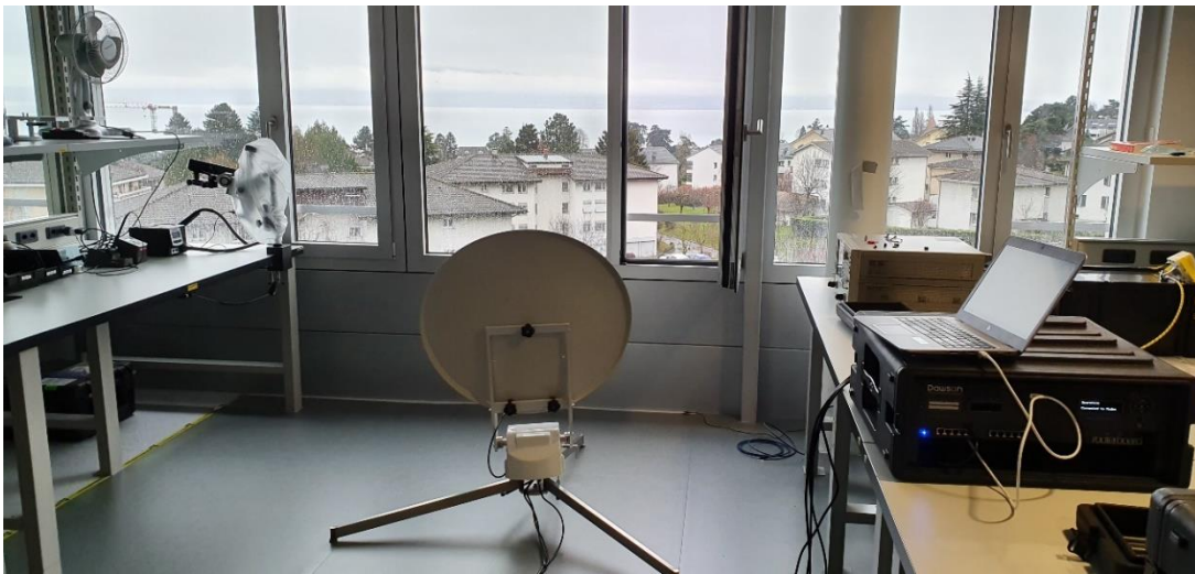
Figure 9 - Dawson SC Zero 70 KA-SAT antenna system in the Viasat lab (powered off)
