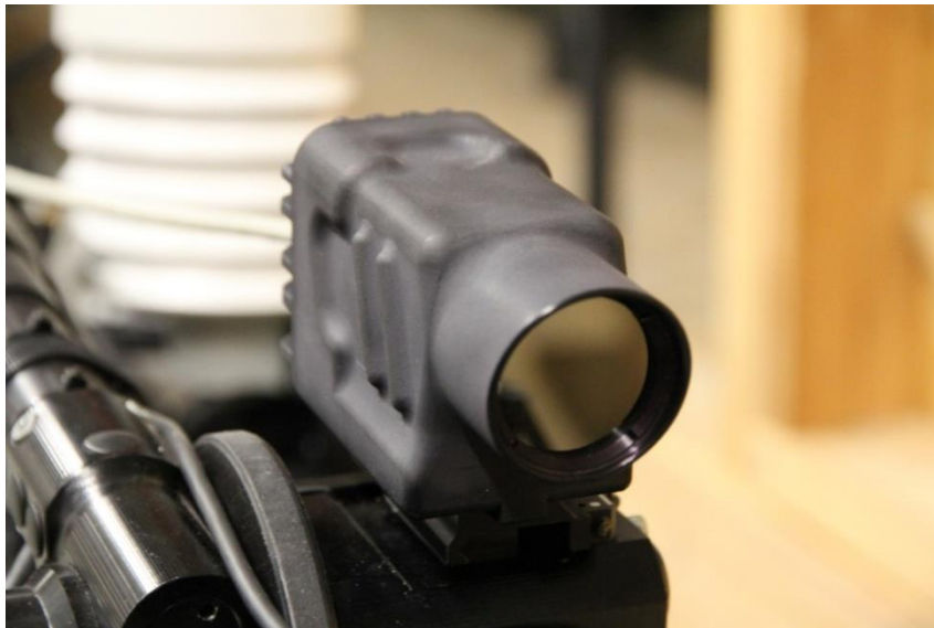
Figure 19 Thermal imaging camera, mounted on the UGV
