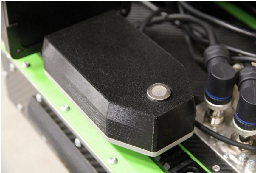
Figure 25 MG-811 sensors, integrated with the UGV
